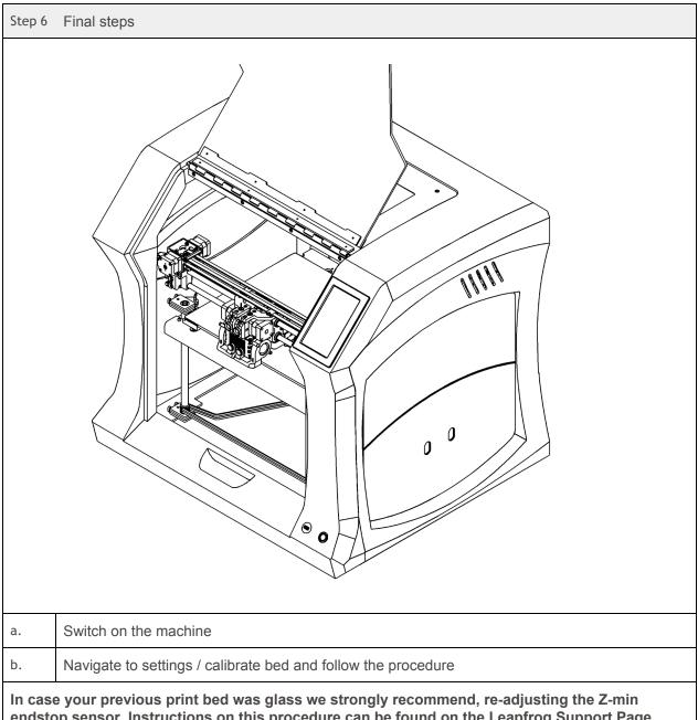
endstop sensor. Instructions on this procedure can be found on the Leapfrog Support Page. Look for Knowledge base / Maintenance / Adjustment: Z-min endstop.
