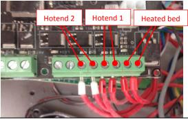
Connect the heating elements to the large connector of the replacement PCB as shown below using the slotted screwdriver (Tool 3):
