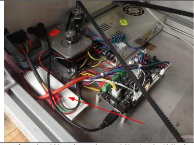
Place the PCB spacers from the old board onto the new PCB using the Philips head screwdriver (Tool 2)
